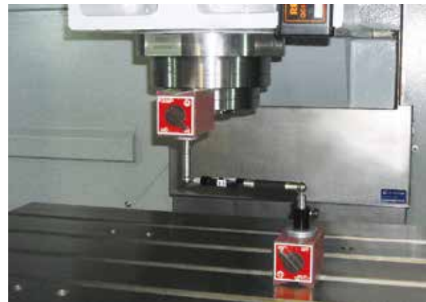
Ball Bar Inspection
